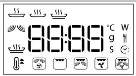
This display shows the clock, the clusters for the 6<sup>th</sup> Sense (5) and Manual (1) cooking functions and the details of all functions, and it helps to adjust all cooking parameters.
