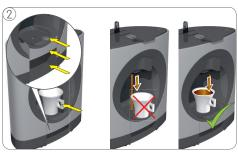
Adjust drip tray position according to the chosen beverage (see page 6-7). Place cup on drip tray.
