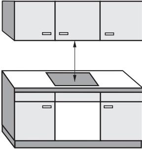
A minimum safety distance must be maintained between the appliance and the cooker hood above it. See the cooker hood manufacturer's operating and installation instructions for details. If the manufacturer's instructions are not available for the cooker hood or if any flammable objects (e.g. utensil rails, wall units etc) are installed above the hob a minimum safety distance of at least 760 mm must be maintained between them and the appliance below.
