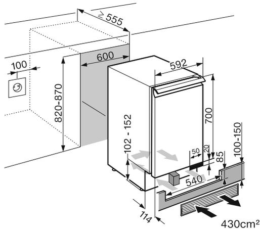
Before installation, ensure the the niche dimensions are the correct size. Before installation, ensure that the ventilation gap dimensions are the correct size. The specified air vents must be observed and the cut-out in the plinth facing must be aligned centrally with the appliance in order to ensure the correct functioning of the wine unit.
