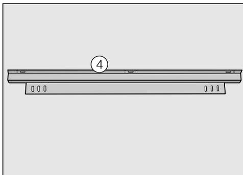
A retaining bracket ④ is required to secure the filler panel. This is available from Miele or from specialist retailers. The retaining bracket can be fitted above or below the wine conditioning unit as required:
