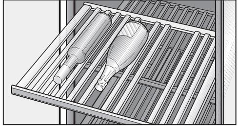
The wooden shelves are on telescopic runners which can be pulled out to make it easier to store and remove bottles.
