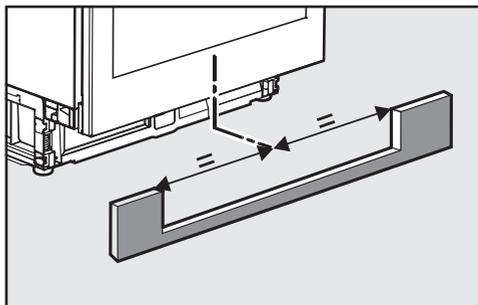
The cut-out in the plinth facing must be aligned centrally with the wine conditioning unit.
