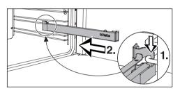
■ Hook the FlexiClip runner onto the front of the lower rail of a side rail (1.) and then push it along the rail into the oven compartment (2.).
