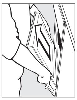
■ Holding the door securely at both sides lift it upwards off the retainers. Make sure you take it off straight.
