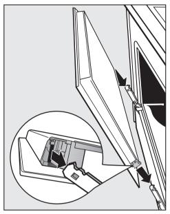
■ Hold the door securely at both sides and carefully fit it back into the hinge retainers.
