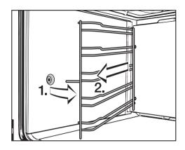
■ Pull the rails out of holder (1) at the front of the oven and then pull them out of the oven (2).
