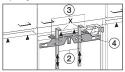
Undo nuts ③ and take fixing bracket ④ off together with fitting aids ②.  Place the furniture door with the outer side downwards on a stable surface.
