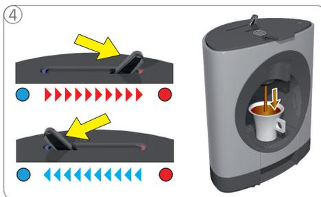
Push selection lever to the "HOT" or "COLD" position as recommended on capsule packs. Beverage preparation starts.
