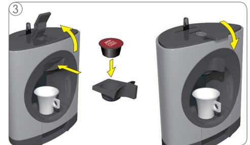
Open locking handle and pull out capsule holder. Insert capsule in capsule holder and insert it back in machine. Close locking handle.
