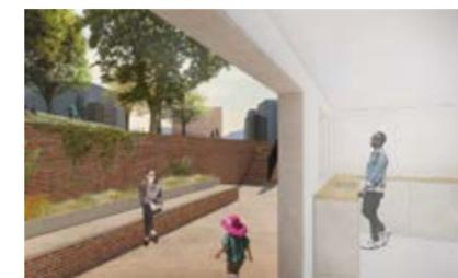
Existing homes could be extended down to basement level and new lightwells formed to bring in light and ventilation
