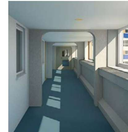
Example of an enclosed deckway
