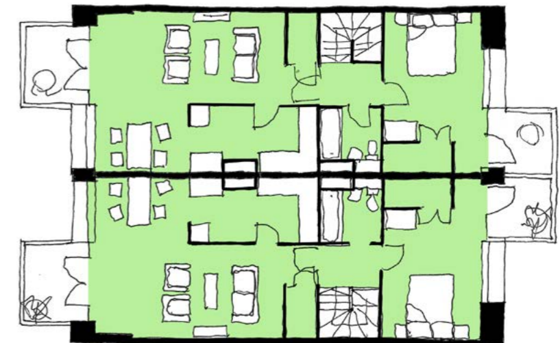
Possible Fourth Floor Plan - addition of insulated skin, living space extended + external projecting balconies
