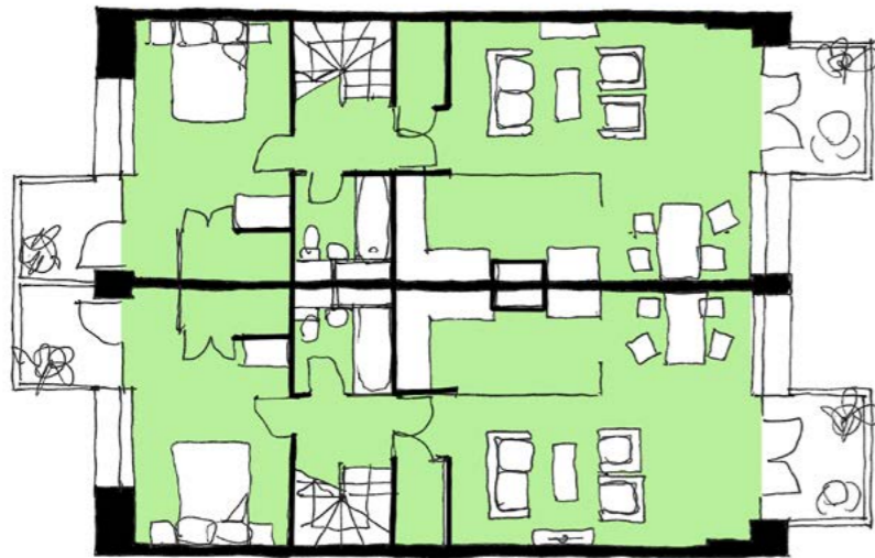
Possible Second Floor Plan - addition of insulated skin, living space extended + external projecting balconies
