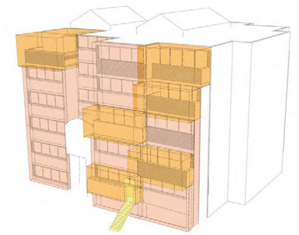
New steps could be added to lower flats to link them to garden level. These could be new front entrances or access to new private gardens for flats formed within the courtyards.
