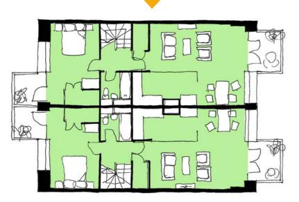
Possible Second Floor Plan - addition of insulated skin, living space extended + external projecting balconies
