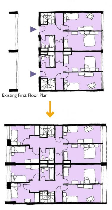
Possible First Floor Plan - addition of insulated skin + extension into existing deck to have 4 bedroom upstairs
