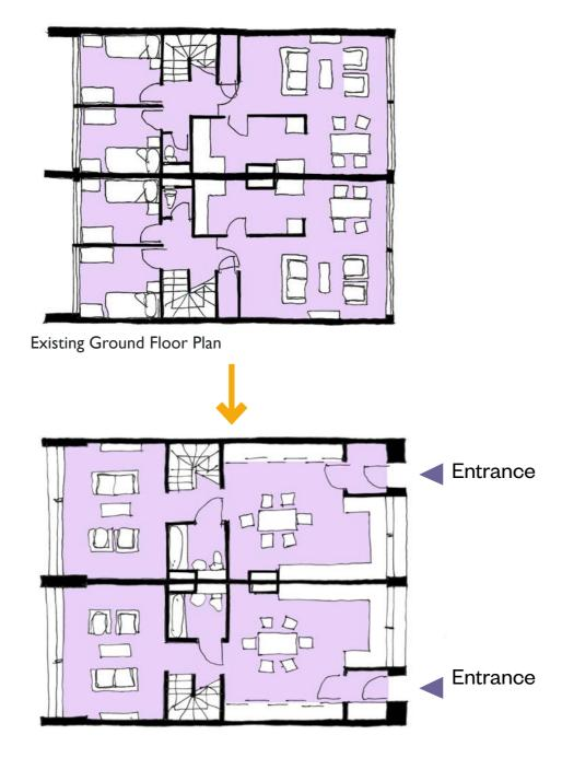
Possible Ground Floor Plan - addition of insulated skin + reconfiguration of internal layout to provide front door entrance
