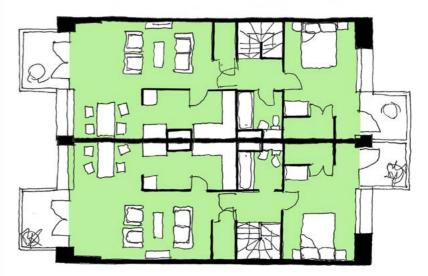
Possible Fourth Floor Plan - addition of insulated skin, living space extended + external projecting balconies
