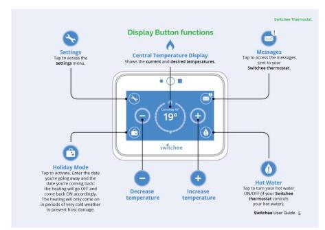
The Switchee smart thermostat also has additional sensors that will help with early detection of damp and mould in your home
