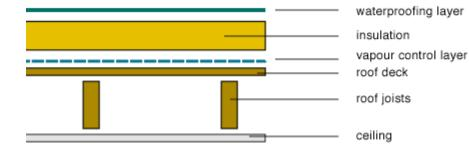
In this building for the flat roof we suggest a warm roof, where all the insulation is located above the structural deck, this avoids the potential risk of condensation within the joist zone. This also allows the easy introduction of the airtightness membrane under the insulation, but on the outside of the roof structure making it possible to do the work without entering the flats.
