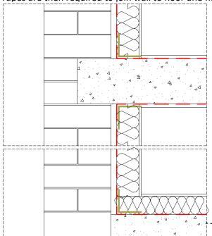
**Red Line** – Denotes position of continuous airtightness barrier. This is formed by the screed and wet plastered walls
