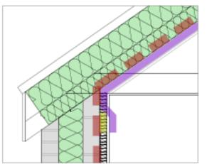
**Red Line** – Denotes position of coninuous air tightness barrier. Use **Covrum 30/30** or **TESCON PROFIL** to seal in corners and around purlins or OSB board.
