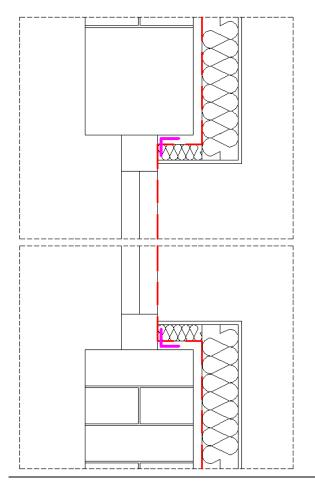
**Red Line** – Denotes position of continuous airtightness barrier, in this case wet plaster and the window.
