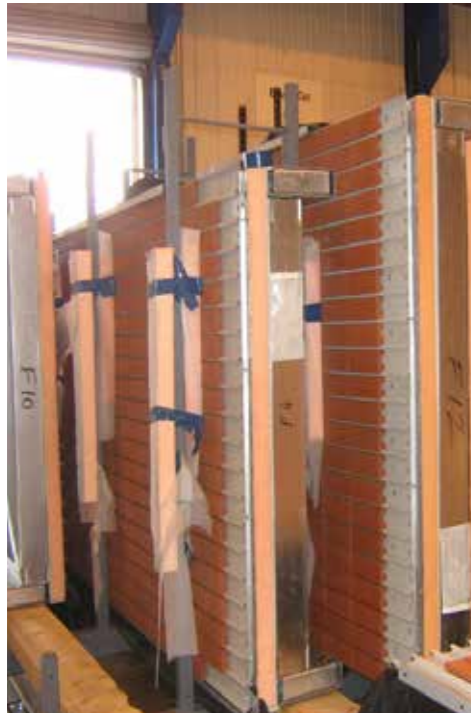
▲ Example of prefabricated brickwork panel manufactured in factory
