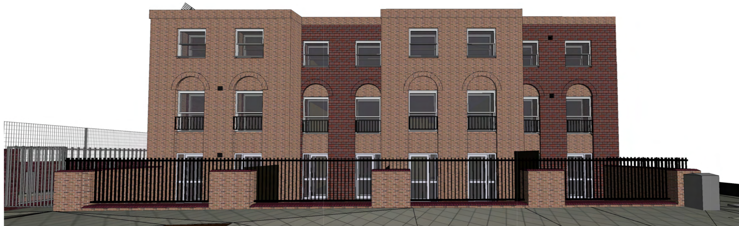
Figure 73 - Design ideas 01- the brickslip over the EWI system is used to match the existing façade color with a contrasting brickslip used to highlight the setback feature.
