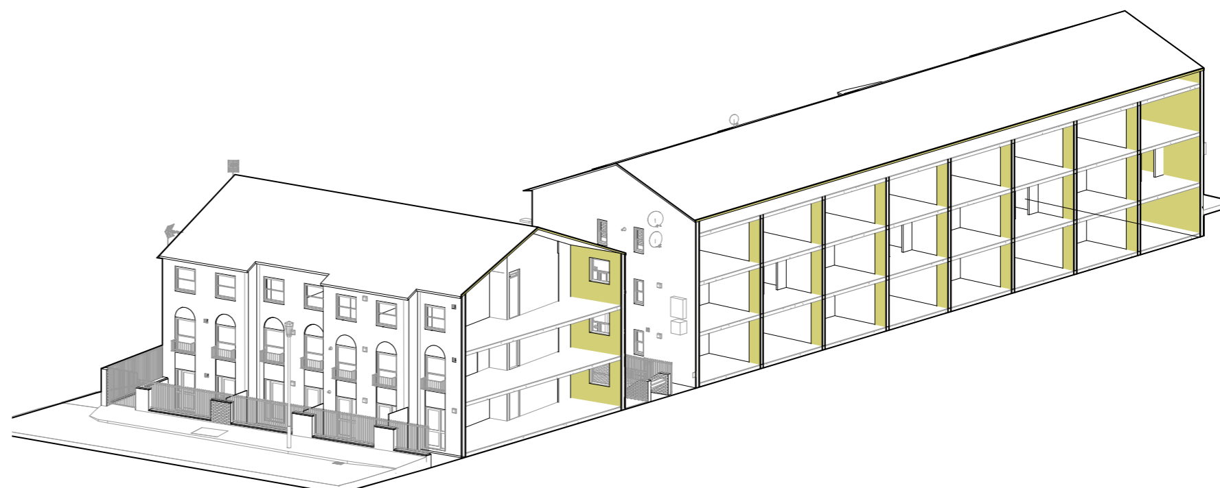
Figure 60 - Axonometric section showing internal wall insulation (IWI)
