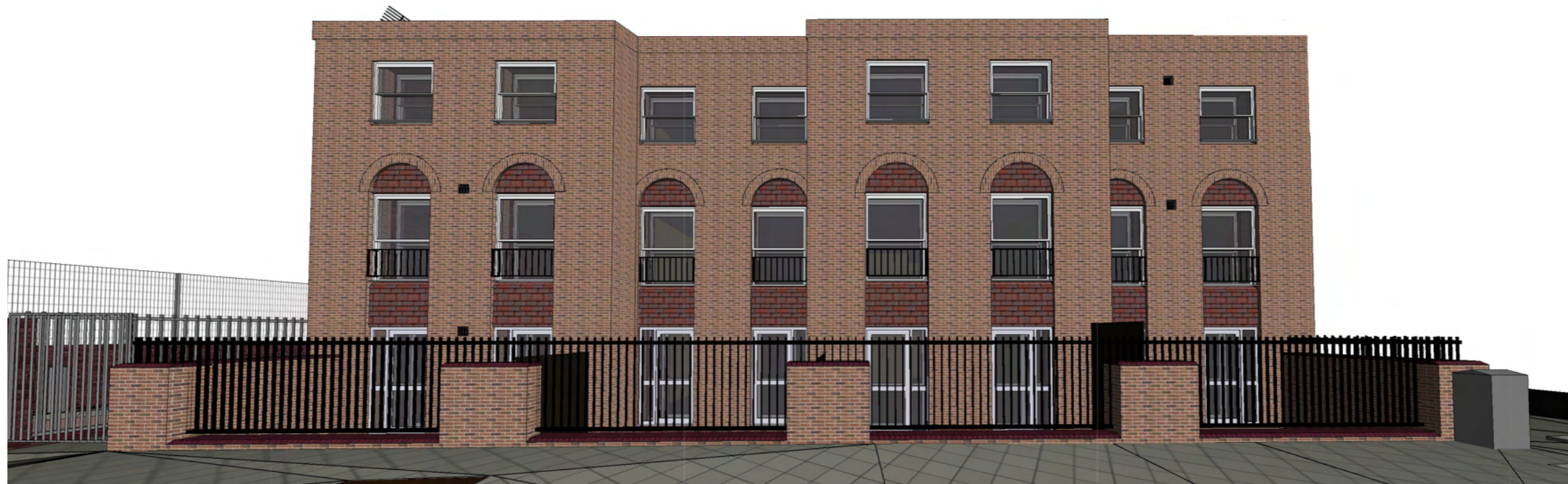
Figure 74 - Design idea 02 – the brickslip is used to emphasise the vertical formation of the existing recess arch windows details along the façade.
