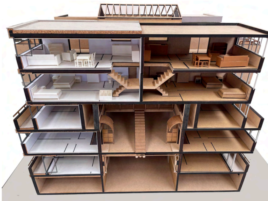
Sectional view of the upper duplexes showing the proposed in white and the existing in brown
