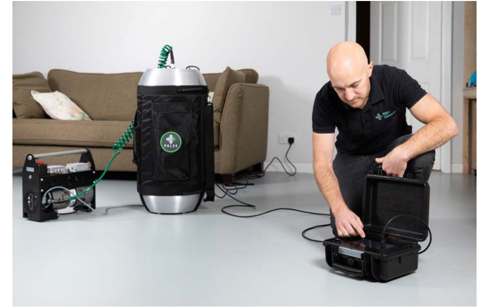
Figure 72 - Airtightness testing using a pulse machine
