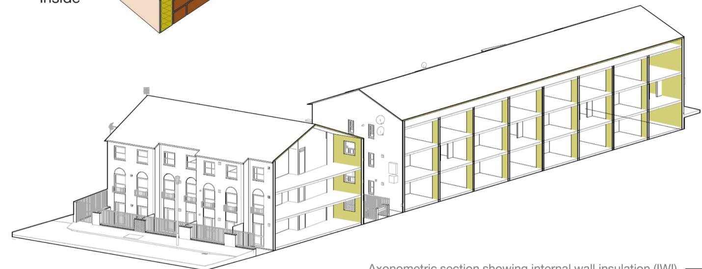
Axonometric section showing internal wall insulation (IWI)
