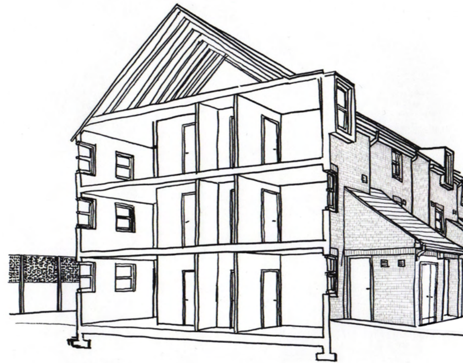
Figure 93 - 3d section of flats with existing entrance, refuse store & gas meter room
