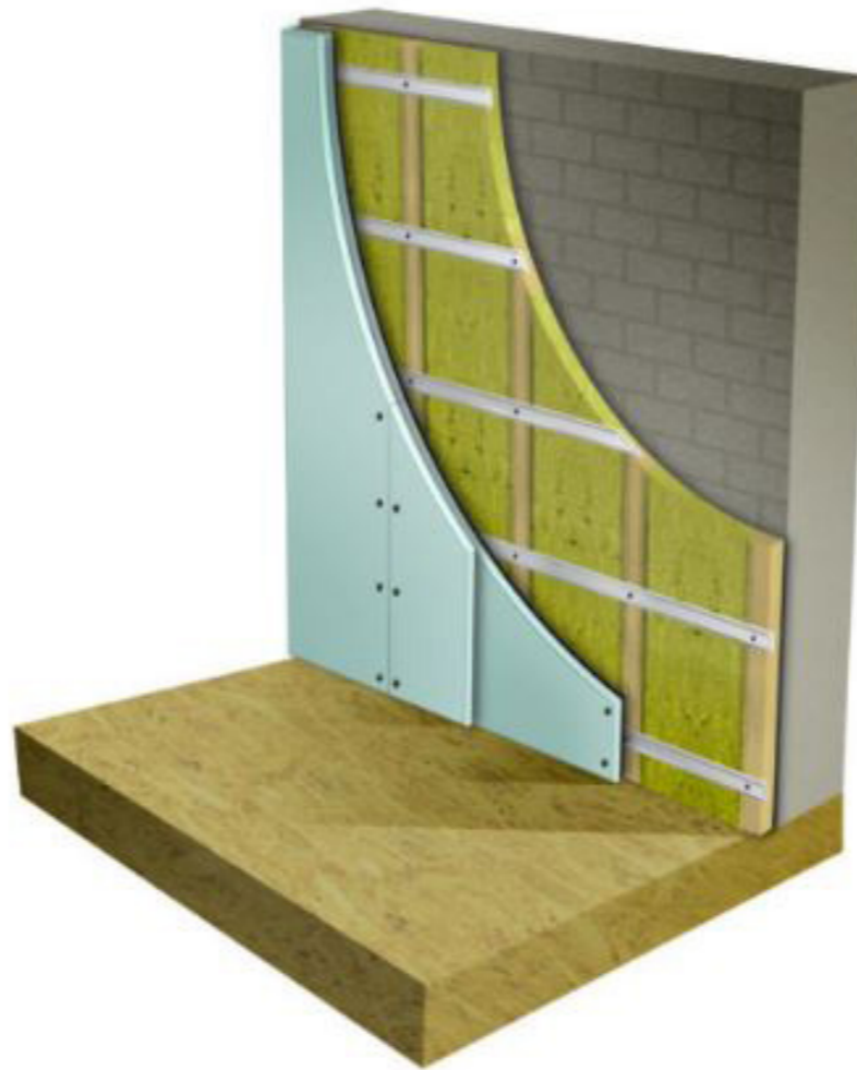
Figure 82 - Example of wall soundproofing system - acoustic insulation, battens and boarding can all be used to stop sound moving through walls
