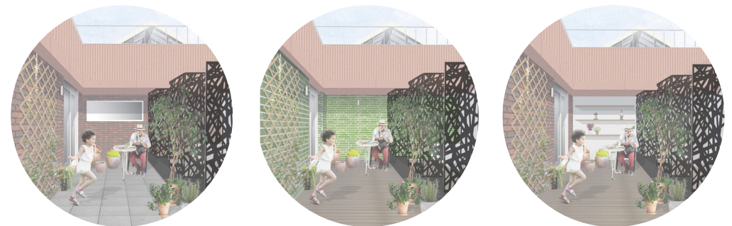
Fire rated glazing New solid screen: brick New solid screen: render finish
