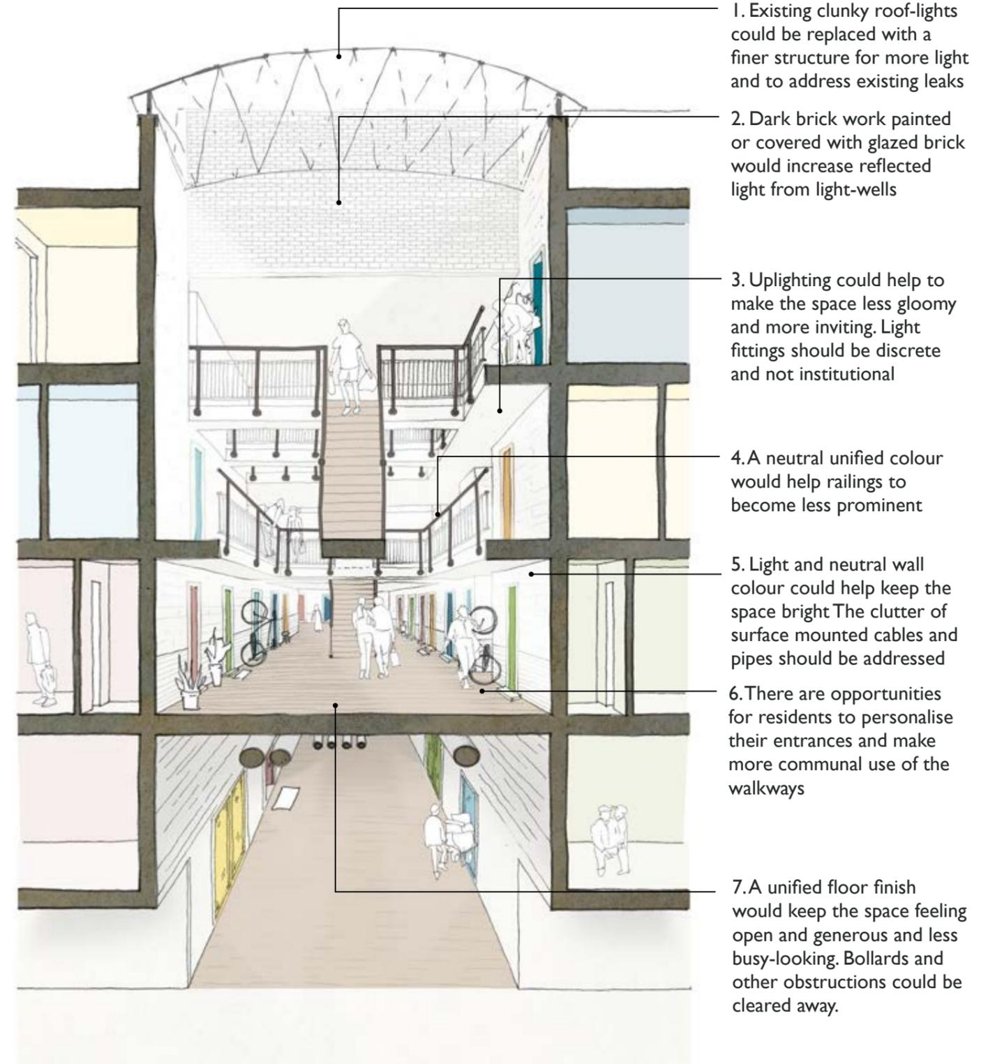
1. Existing clunky roof-lights could be replaced with a finer structure for more light and to address existing leaks
