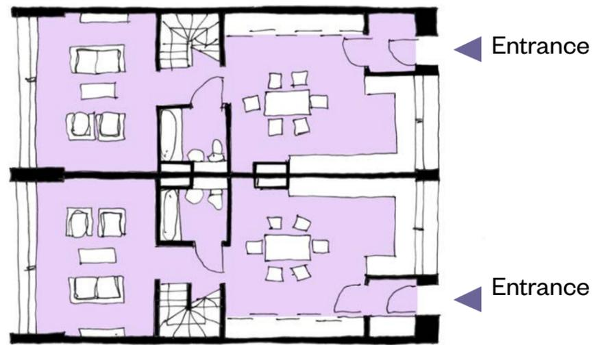
Possible Ground Floor Plan - addition of insulated skin + reconfiguration of internal layout to provide front door entrance
