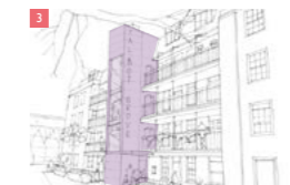
New lift & defined main entrance.
