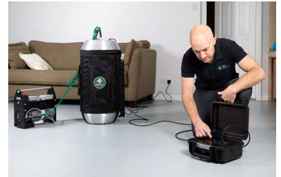
Figure 25 - Airtightness testing using a pulse machine
