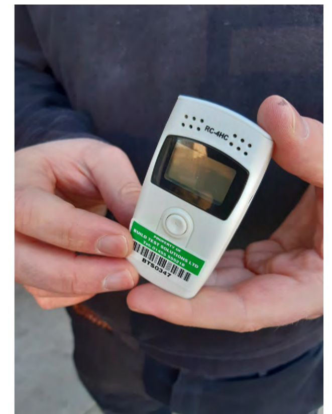
Figure 26 - Monitoring device used to calculate Heat Transfer Coefficient
