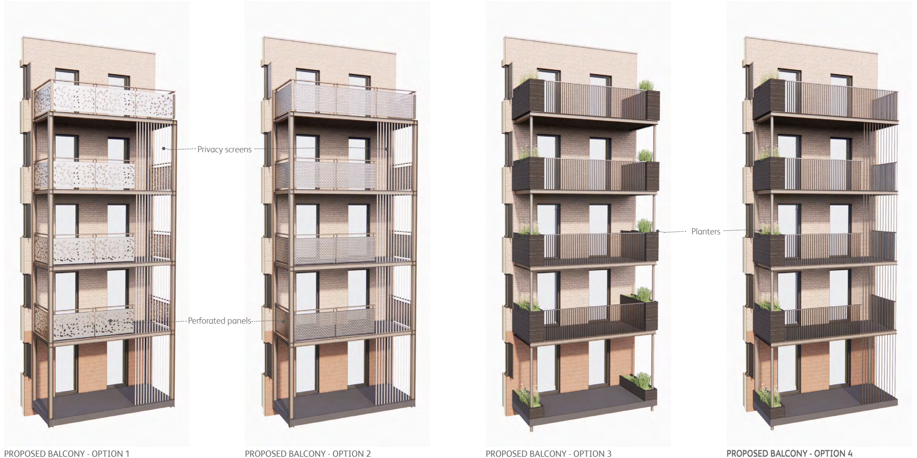
Figure 90 - Structural & Finish possibilities for west facing balconies
