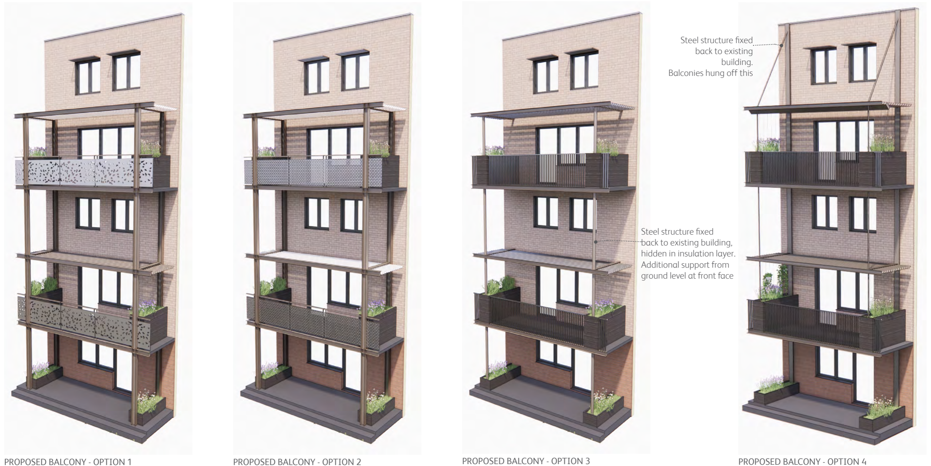
Figure 89 - Structural & Finish possibilities for south facing balconies
