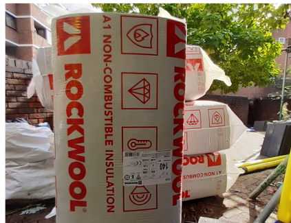
Figure 15 - Mineral wool insulation to go in the roof
