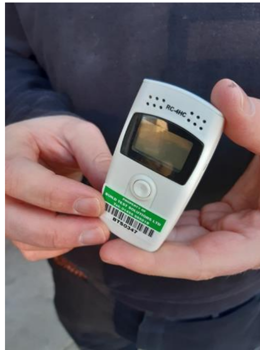
Thermal and Humidity sensors
