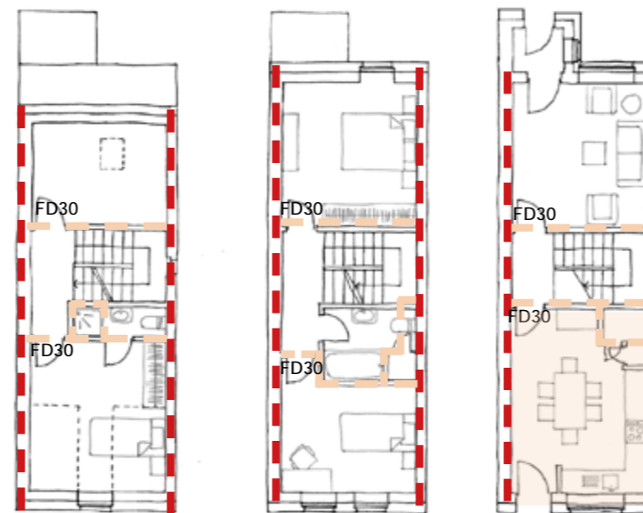
SECOND FLOOR FIRST FLOOR GROUND FLOOR
