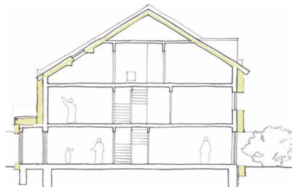
Figure 37 - External wall insulation in section
