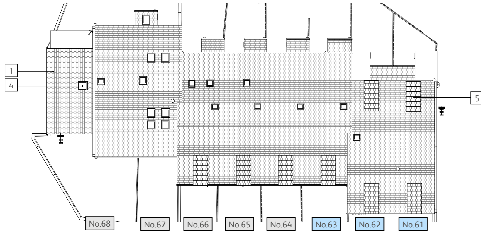
Figure 23 - Block 06 - Existing Roof Plan
