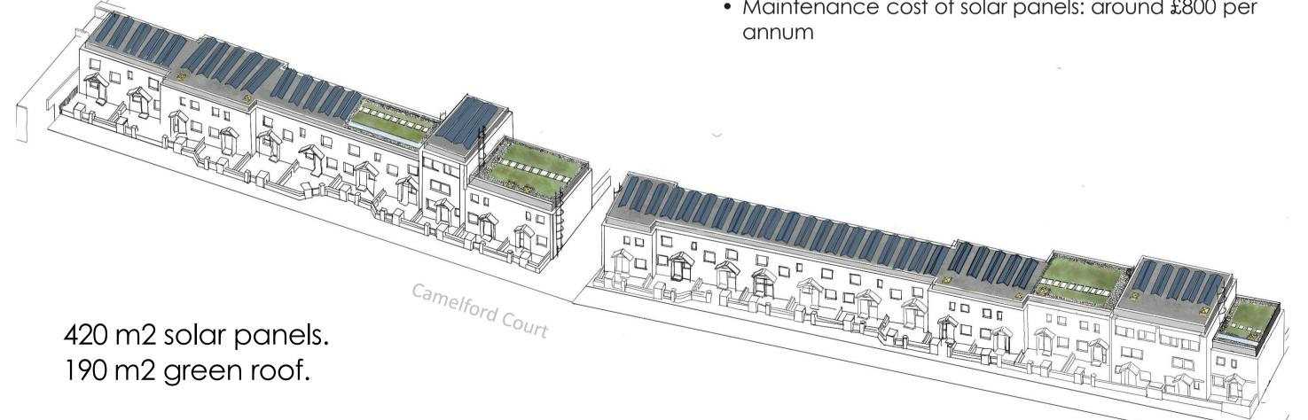
Design Option 01 Maximum solar PV panels: 69:31 Solar Panels to Green Roof Clarendon Road
