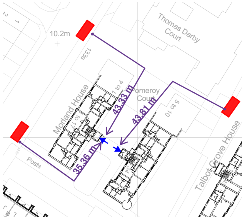
Figure 10.1 – Fire vehicle access to Morland House
