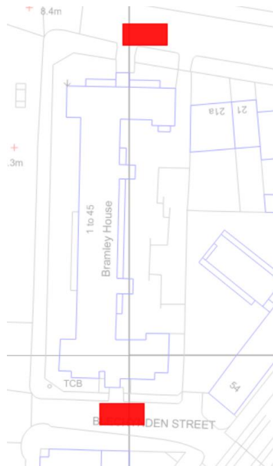
Figure 14.2 – Fire vehicle access to Bramley House
