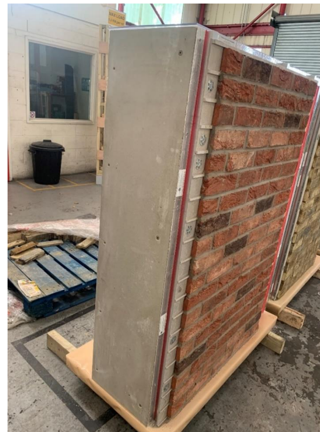
Example of an external wall insulation system using brick slips
