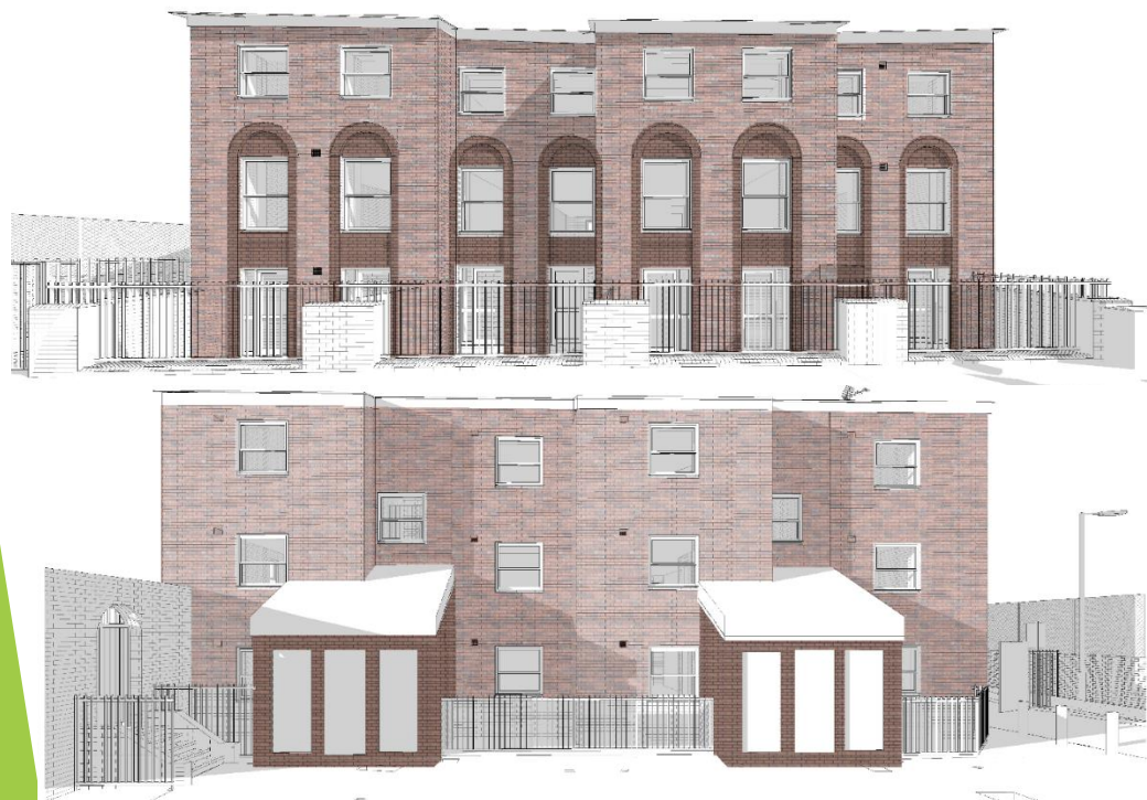
Option 01: Use of a multi red brick finish similar to existing with zones of contrasting brick slip to highlight façade features
