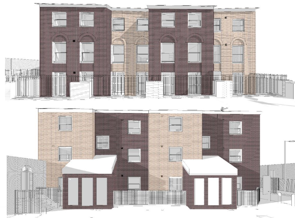
Option 02: Combinations of 2 brick finishes highlighting the different setbacks along the façade.
