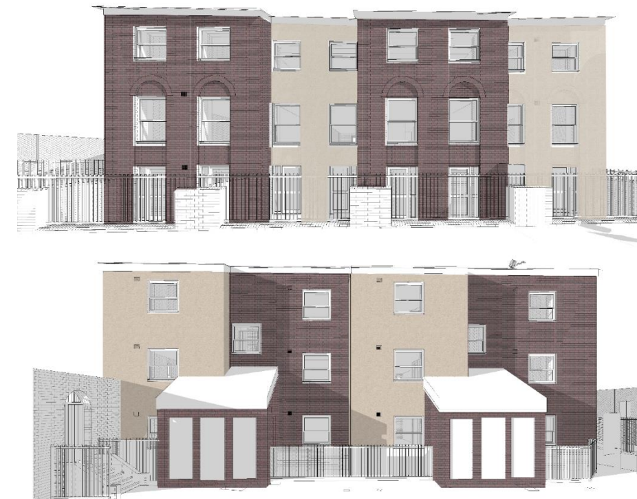
Option 03: Combinations of brick and render finishes highlighting the different setbacks along the façade.
