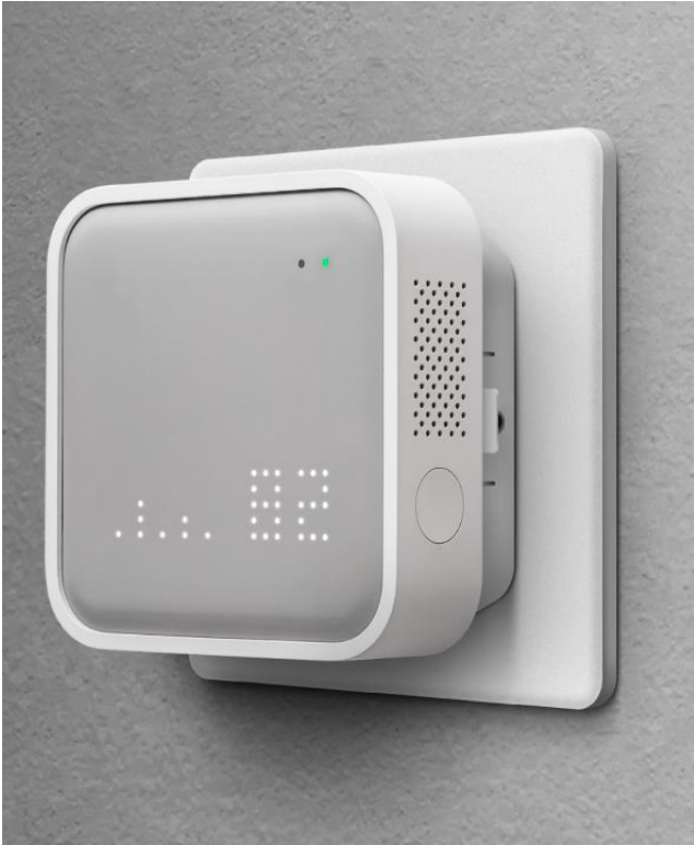
Awair internal air quality monitors included as part of green skills equipment library
