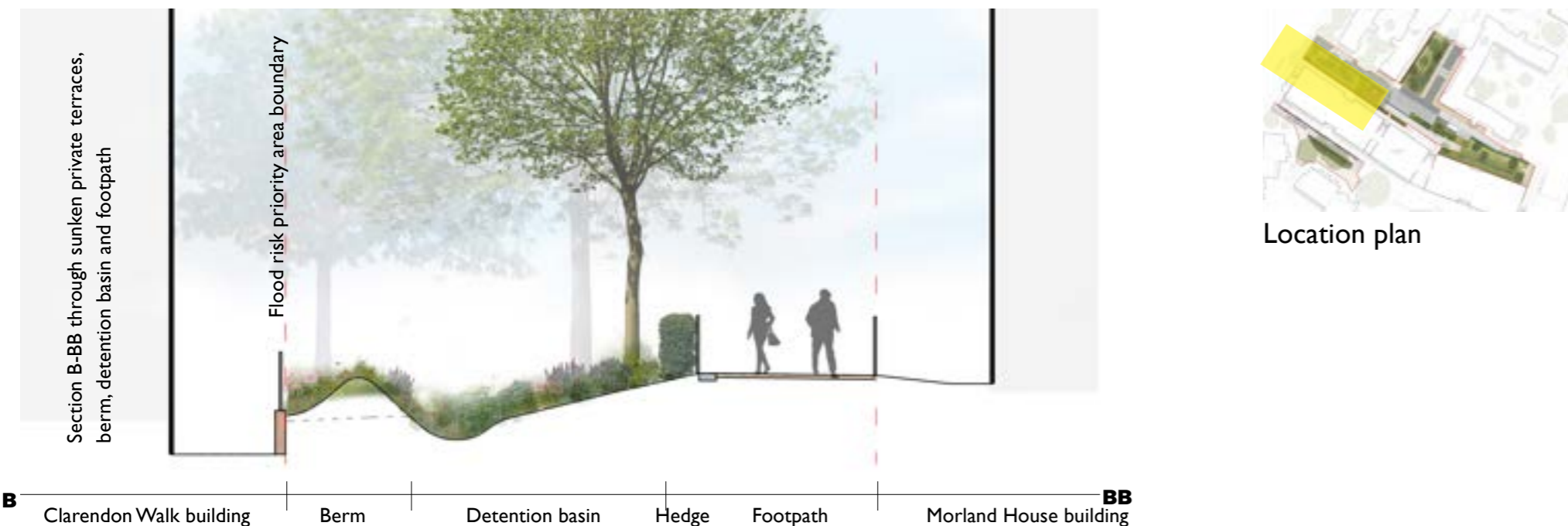
Zoom in of area 2 - detention basin and berm
