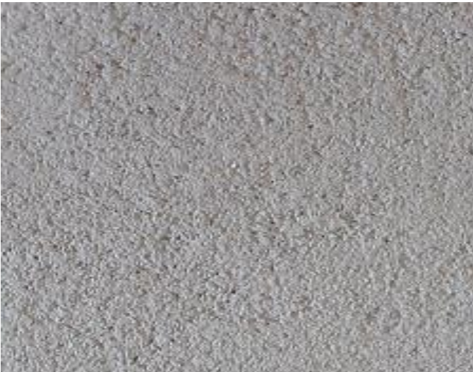
Light grey render 'Accent' – to balcony back walls, piers between windows and other areas
