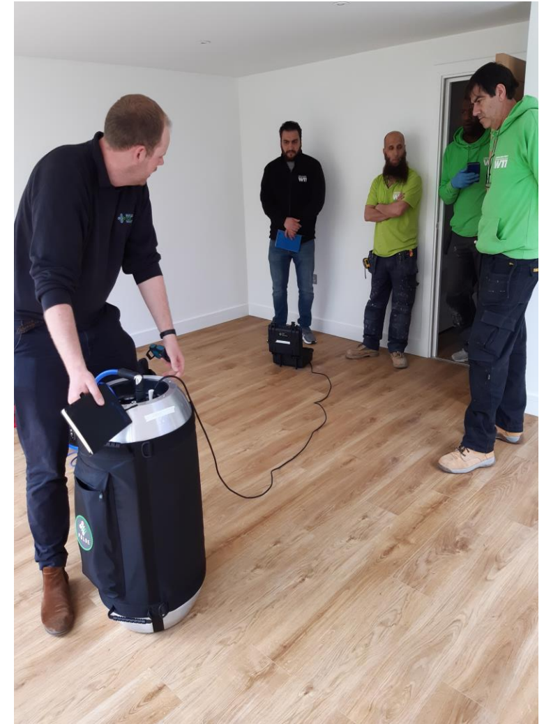
Image 11: a picture of the Lancaster West Neighbourhood Team's Repairs Team learning how to do pulse air tightness tests to check the energy efficiency of residents' properties.
